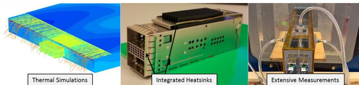
Figure 6: Extensive thermal modeling, design and testing has been performed on the QSFP-DD to validate thermal performance
