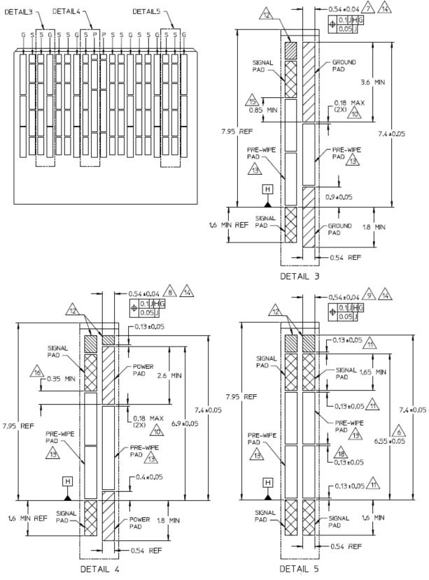
Figure 17: Module pad dimensions
