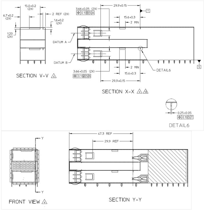
Figure 20: 2x1 stacked cage dimensions
