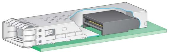
Figure 25: SMT connector in 1xn cage
