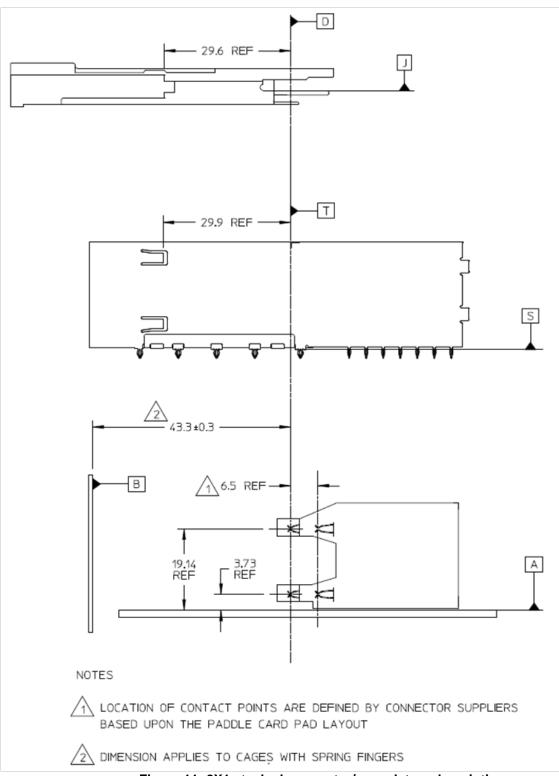
Figure 11: 2X1 stacked connector/cage datum descriptions
