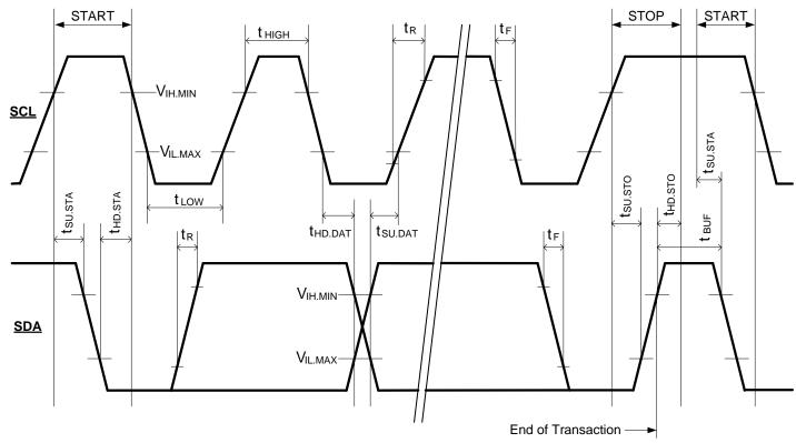
Figure 37: QSFP-DD Timing Diagram
