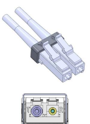
Figure 35: Dual LC optical patchcord and module receptacle
