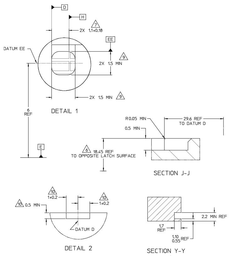
Figure 15: Detailed dimension of module
