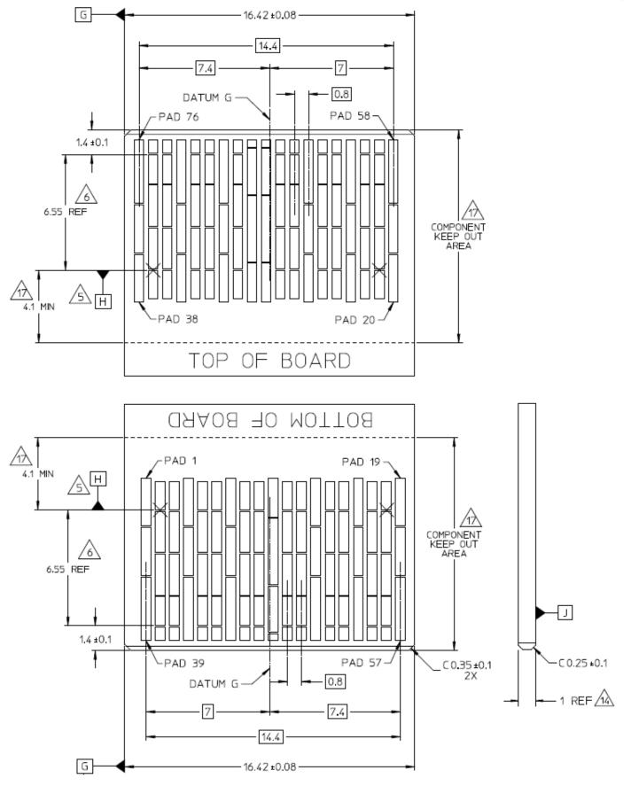
Figure 16: Module paddle card dimensions
