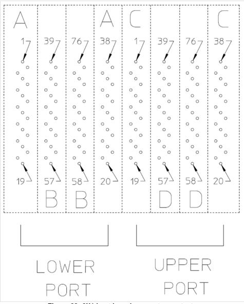
Figure 23: 2X1 host board connector contacts
