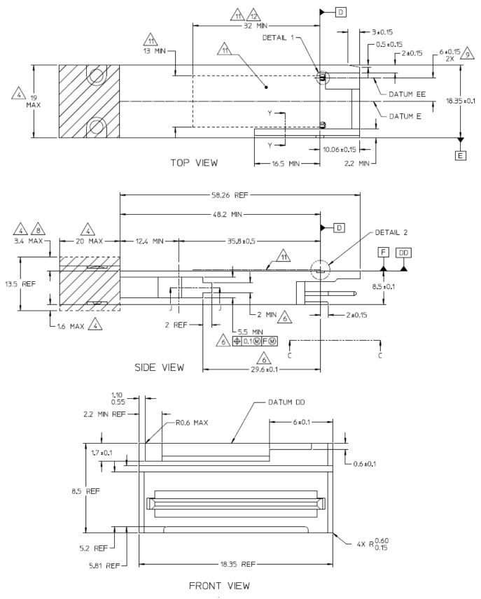
Figure 14: Drawing of module
