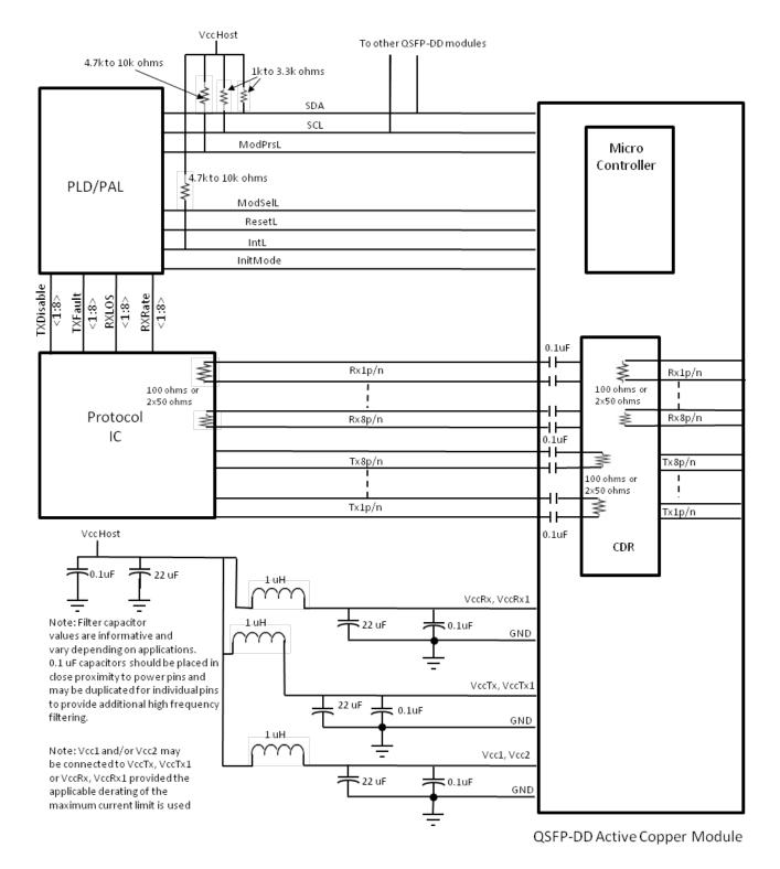
Figure 4: Example QSFP-DD Host Board Schematic for active copper cables
