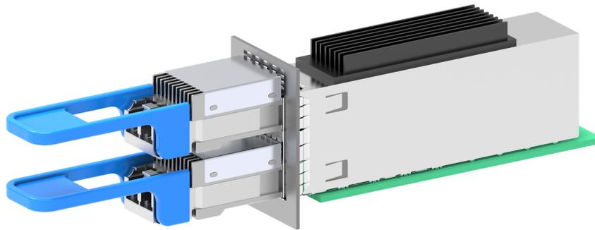
Figure 2-8: Two type 2B modules shown in a QSFP-DD800 stacked cage. Note the alignment of the faceplate and cage openings coincide with the nose heatsink channels
