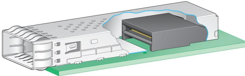
Figure 2-4: Surface mount connector in a 1x1 cage
