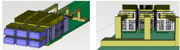
Figure 5-4: Stacked 2x1 cage with cabled upper port
