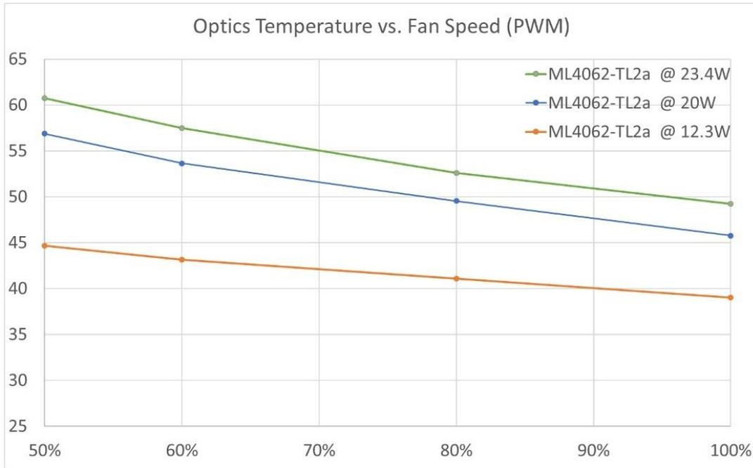
Figure 6-5: Average temperature optics module (MultiLane ML4062-TL2a DD Module) in 1RU chassis vs fan speed, chamber temperature is 25°C
