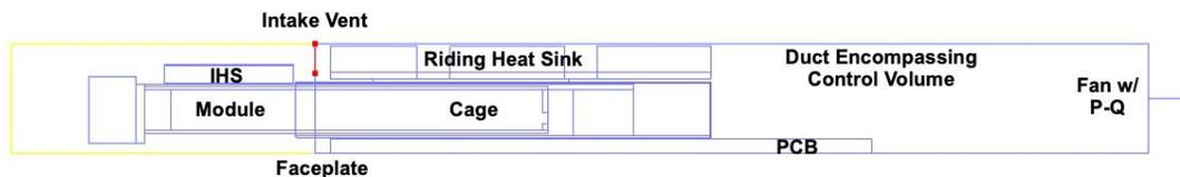
*Fig 3-1: Boundary conditions for module-level analysis*
