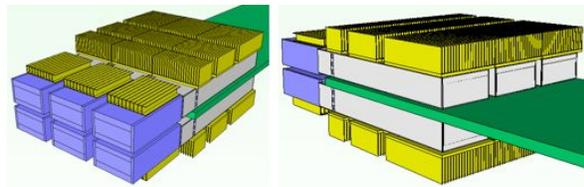
Figure 5-6: 1x1 cage implemented in a belly-to-belly configuration
