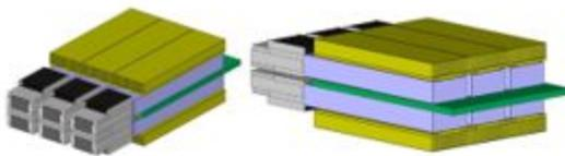
Figure 5-7: 1x1 alternate cage implemented in a belly-to-belly configuration
