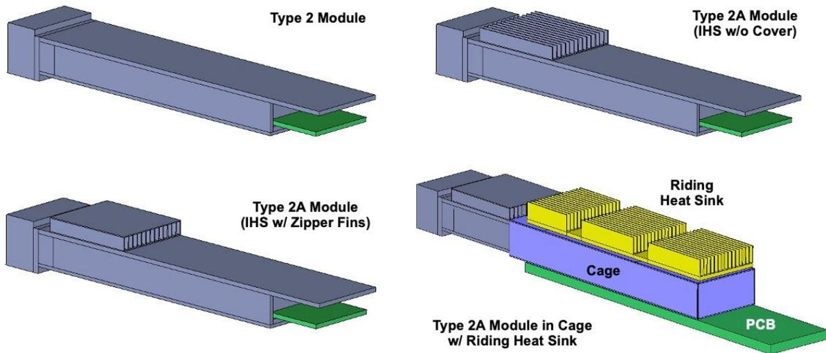
Figure 3-2: Thermal models of module types simulated
