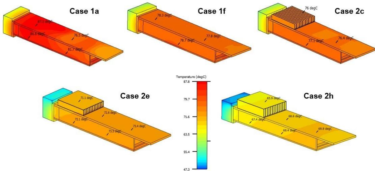
Figure 3-4: Surface temperature map of module housing for select cases
