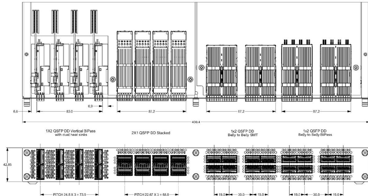
*Figure 5-8: Experimental configurations showing the top view and front view of the four cage configurations under test*
