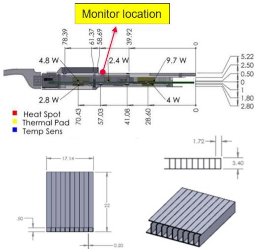
Figure 5-1. Details of the thermal module used; when a Type 2A module is used, the nose heatsink is implemented as depicted
